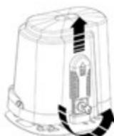
Release the motor (turn the key counter clockwise until the limit is reached without forcing) and move the gate by hand.
